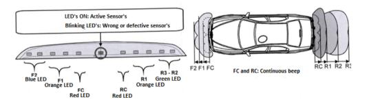
**Technical specification** Power supply; 9 - 24V Active current consumption of sensors; 120mA max Operating temperature; -25 / + 70 ° C
